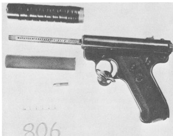
FIG. 5—Group III silencer. The expansion chamber screws over the distal end of the barrel so that the bullet remains in the barrel throughout its course through the weapon. (AFIP Negative 78-4649-5.)
