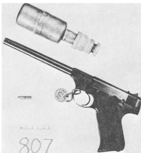
FIG. 2—Group II silencer. The front sight has been removed from the weapon, and the silencer is held in place simply by friction fit. (AFIP Negative 78-4649-2.)
