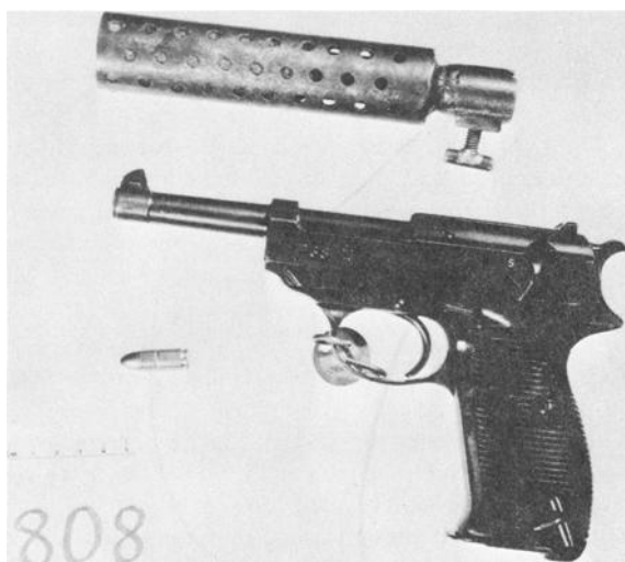
FIG. 1—Group I silencer. The silencer is held in position by the thumbscrew. (AFIP Negative 78-4649-1.)
